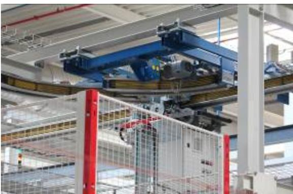
*BU: Wide variety of solutions for factory and logistics automation: Conductor rail system 0815 in an Electrified Monorail System*
