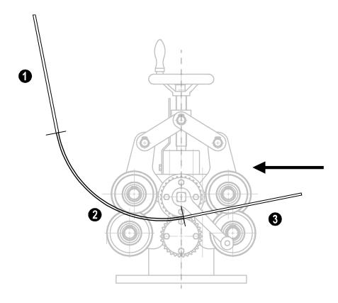
4. **Loosen** the spindle, pull the rail out.
