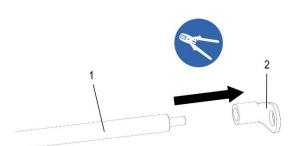
Fig. 134: Crimp equipotential bonding cable with crimping cable lug
