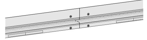
Fig. 81: Fully mounted connection point of rails without offset
