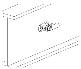
Fig. 85: PE connector seated in elongated hole
