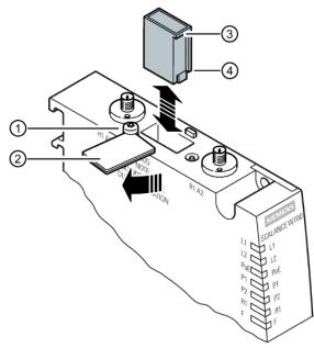
Fig. 190: Replace WLAN transceiver using removable media (Key/C-plug) (source: Siemens Operating Manual C79000-G8900-C325-15 page 62)
