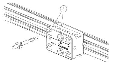
Fig. 94: Drill 2 holes for PE connection
