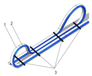
Fig. 132: Laid cables with cable ties
