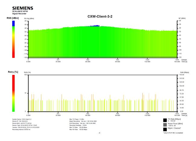
Fig. 203: Signal scan with low retry rate and constant WLAN data rate (150 Mbps)
