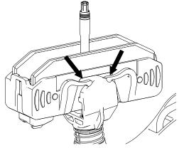
Fig. 179: Correct position of springs
