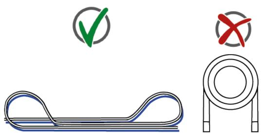
Fig. 133: Loop formation is allowed; coil winding prohibited
