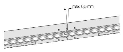
Fig. 82: Maximum offset of connection point in X-direction (direction of travel)
