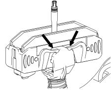
Fig. 165: Correct position of springs
