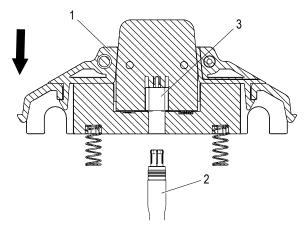
Fig. 180: Collector housing (1) is mounted on data cable (2)
