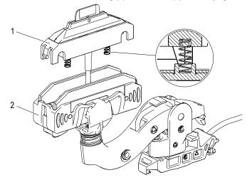
Fig. 182: Collector housing (1) is mounted on balance (2)
