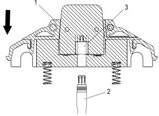
Fig. 166: Collector housing (1) is mounted on data cable (2)
