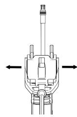
Fig. 152: Disassemble balance incl. sliding contact from joint
