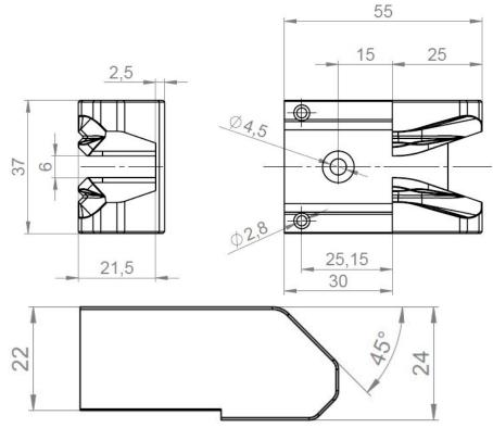
Fig. 118: Aluminium transfer guide
