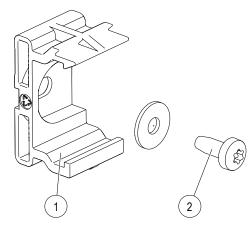
Fig. 37: Hanger clamp with self-tapping screw
