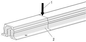
*Fig.* 97: Shorten ProfiDAT<sup>®</sup> compact rail (with positioning strip)
