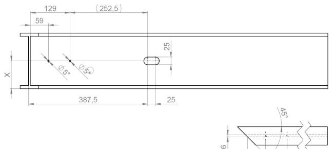
Fig. 123: Drill hole positions for end feed with single expansion unit with aluminium overrun cap (45° cut on long side of substructure (support structure))
