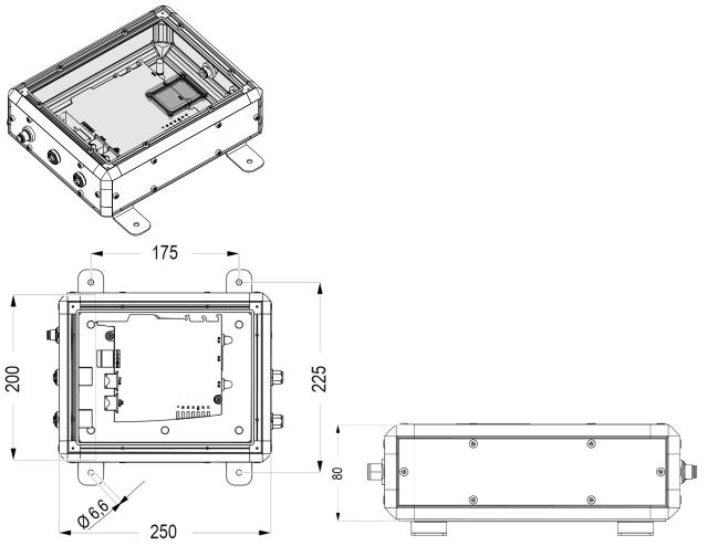
Fig. 3: Transceiver housing dimensions and illustration
