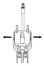
Fig. 175: Disassemble balance from joint
