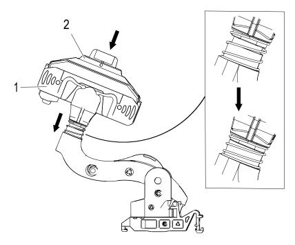
Fig. 189: Check collector head in installed state
