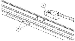
Fig. 95: Tighten the 2 self-tapping screws
