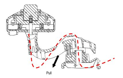
Fig. 149: Pull data cable (HF cable) (loop from below)
