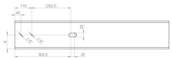
Fig. 120: Drill hole positions for end feed with expansion unit and aluminium overrun cap
