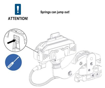
Fig. 150: Carefully press nose in collector housing inward with flat-head screwdriver
