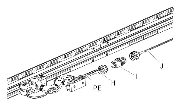
Fig. 142: Connection to mobile antenna
