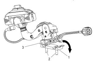
Fig. 124: Mount collector on towing unit
