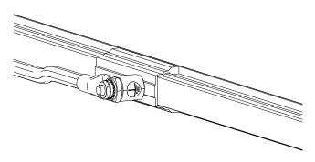
Fig. 93: PE connector is mounted
