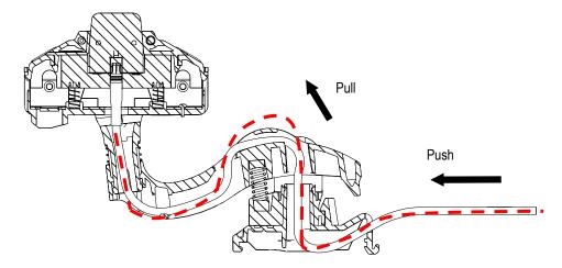
Fig. 171: Pull data cable (HF cable) (loop from above)
