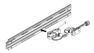
Fig. 125: Slide collector into rail
