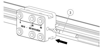
Fig. 88: Step drill M3 90° into lateral drill hole
