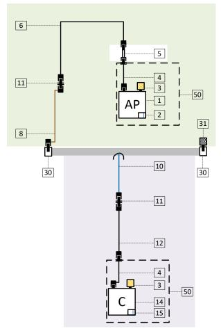
Fig. 30: Overview and arrangement of the electrical components. Example: End feed, client with one antenna, without additional housing, equipotential bonding not shown
