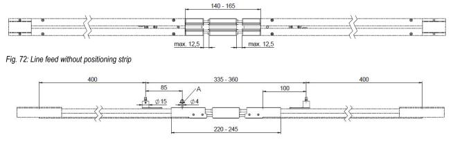
Fig. 73: Line feed without positioning strip; A = anchor point
