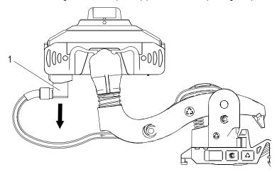
Fig. 170: Pull off angled blade receptacle
