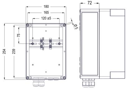
Fig. 4: Polycarbonate housing dimensions and illustration
