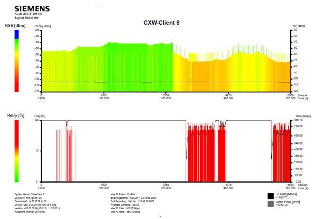
Fig. 204: Signal scan with too low signal strength, resulting in many retries and data rate drop
