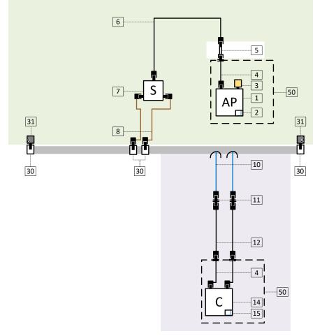
Fig. 29: Overview and arrangement of electrical components. Example: Line feed, client with two antennas, without additional housing, equipotential bonding not shown
