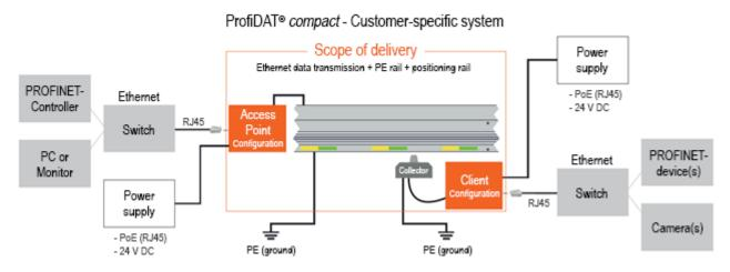
Fig. 1: Overview of interfaces and scope of delivery ProfiDAT<sup>®</sup> compact (simplified)
