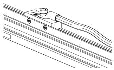
Fig. 96: PE connection is mounted
