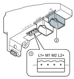
Fig. 145: Transceiver connection for Ethernet
