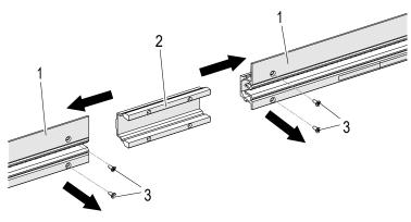
Fig. 70: Disassemble connector
