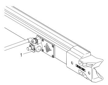
Fig. 139: Line feed to stationary antenna
