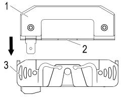
Fig. 160: Insert sliding contact (1) into balance (3)
