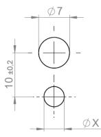
Fig. 38: Distance between drill holes in support structure (substructure) for hanger clamp
