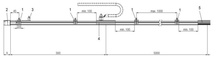
Fig. 33: Minimum and maximum distances between hanger clamps
