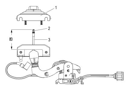
Fig. 174: Disconnect collector housing (1) from data cable (HF cable) (3)
