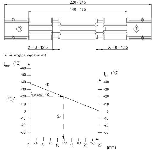
Fig. 55: Determine air gap
