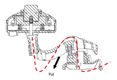
Fig. 172: Pull data cable (HF cable) (loop from below)
