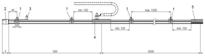
Fig. 39: Minimum and maximum distances between hanger clamps
