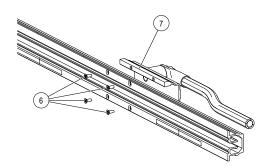
Fig. 92: Tighten all 4 self-tapping screws
