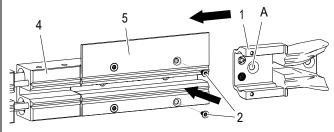
Fig. 64: Mount transfer guide
