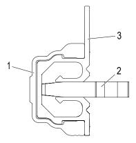
Fig. 77: Mount connector onto ProfiDAT®compact rail
