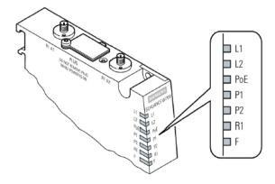
Fig. 191: Transceiver LED state (Source: Scalance W774-1 / W734-1 Operating Instructions)
