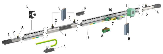
Fig. 15: ProfiDAT® compact components in detail
