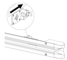
Fig. 25: End feed with stationary antenna
