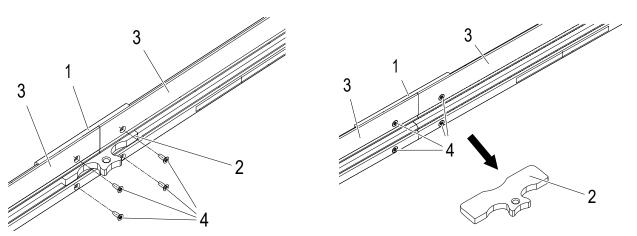
Fig. 79: Tighten 4 self-tapping screws (2 Nm)
