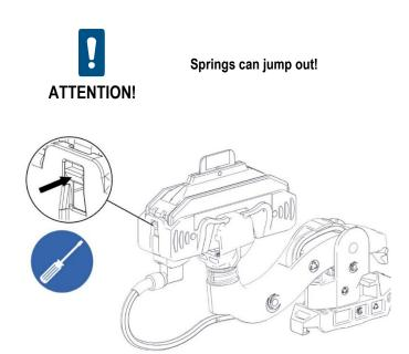
Fig. 173: Carefully press nose in collector housing inward with flat-head screwdriver
