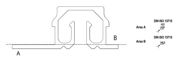
Fig. 99: Deburr ProfiDAT<sup>®</sup> compact rail
