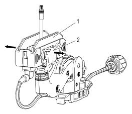
Fig. 176: Balance incl. sliding contact (1) and joint (2)
