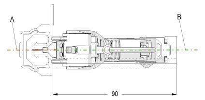
Fig. 127: Collector mounting dimension from towing unit to bottom edge of rail
