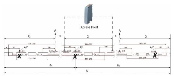
Fig. 51: Expansion unit dimensioning on segment
