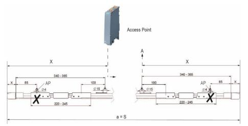
Fig. 53: Expansion unit layout at end
