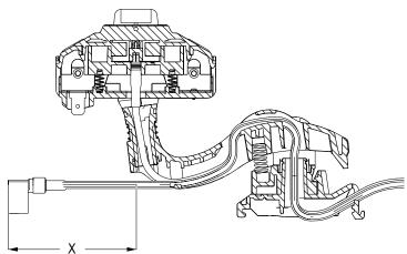
$\rightarrow$  Check the length of the PE cable (x = 120 mm) (see Fig. 186).
