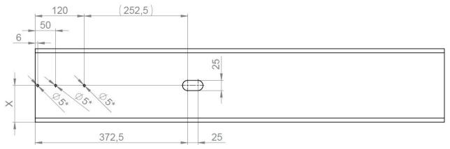
Fig. 121: Drill hole positions for end feed with expansion unit and plastic overrun cap
