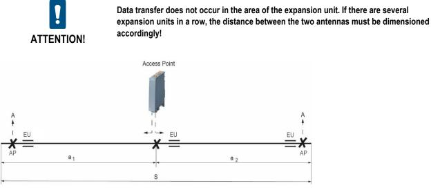
Fig. 50: Expansion unit dimensioning on segment
