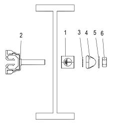
Fig. 84: Mount PE connector onto support structure (substructure)
