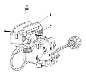
Fig. 153: Balance incl. sliding contact (1) and joint (2)
