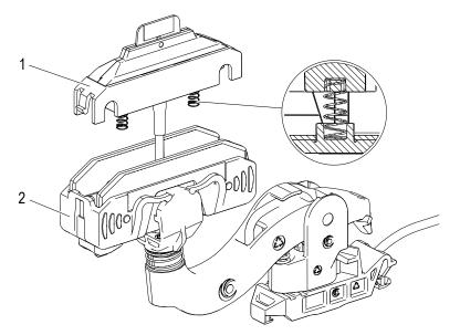
Fig. 168: Collector housing (1) is mounted on balance (2)
