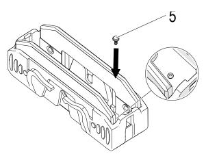
Fig. 162: Tighten STS-plus 1.4x4 – T5 screw
