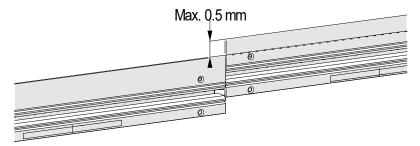
Fig. 83: Maximum offset of connection point in Y-direction
