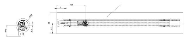
Fig. 49: Support structure (substructure) (1) with line feed (aluminium cap, left)
