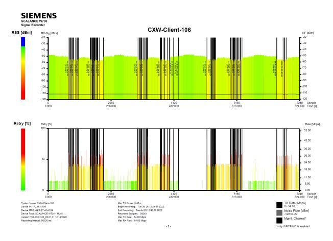
Fig. 202: Multiple crossing of same segment transfer with incorrect roaming processes (multiple vertical black lines in transfer area)
