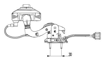
Fig. 126: Screw distances in towing unit
