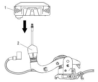
Fig. 163: Balance incl. sliding contact (1) is mounted
