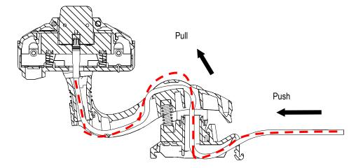
Fig. 148: Pull data cable (HF cable) (loop from above)
