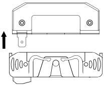
Fig. 158: Loosen STS-plus 1.4x4-T5 screw
