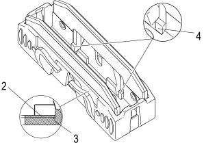
Fig. 161: Copper plate (2) of sliding contact is centered on bottom of balance (3)
