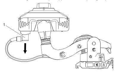
Fig. 147: Pull off angled blade receptacle
