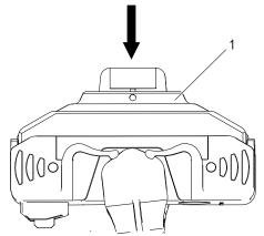
Fig. 185: Check collector housing ease of movement
