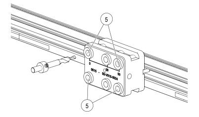
Fig. 91: Drill 4 holes for PE connector
