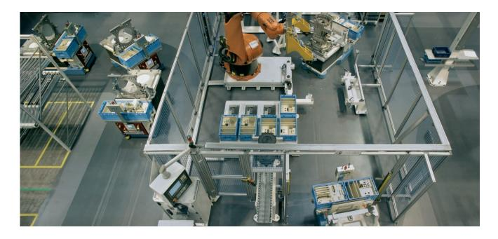
For floor surface conveyors, the goal is to achieve a level floor with no obstacles for persons, forklifts or other equipment in the factory environment, to eliminate hazardous contact rails, and to render batteries in vehicles either superfluous or more efficient.
