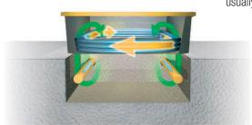
The secondary Pickup is able to move freely. It can be positioned with an air gap and sufficient tolerances in relation to the primary conductors and can also move at any speed.
