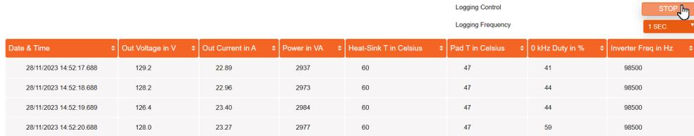
→ The [Stop] button appears under 'Logging Control' while recording is in progress. Click on the [Stop] button.
