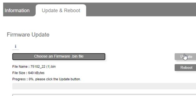
6. In Bootloader mode, the name and size of the selected bin file is displayed under the [*Choose a firmware .bin file*] button. Click on the [*Update*] button.
