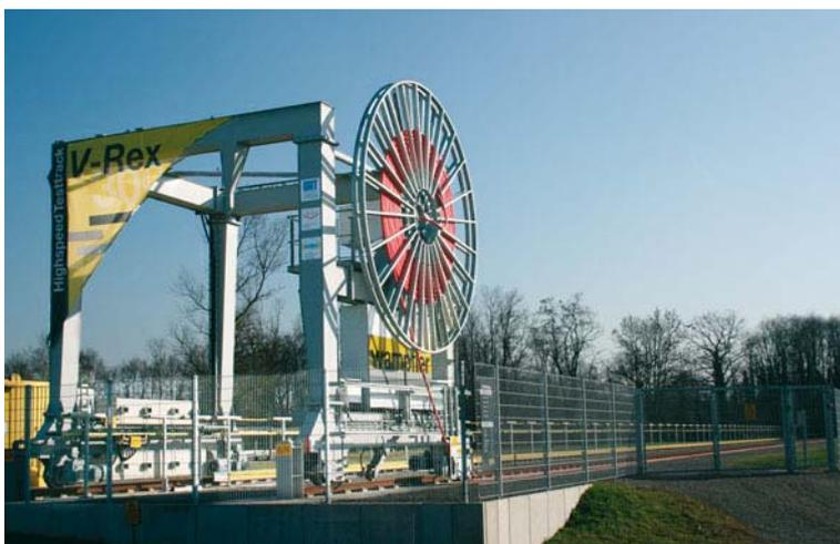
*Caption: A nearly authentic and therefore ideal testing area: Testtrack V-Rex on the premises of Wampfler AG in Weil am Rhein with a velocity of up to 300 meters per minute and a traverse path of up to 140 meters. A real load test for motor reels with medium voltage cables.*
