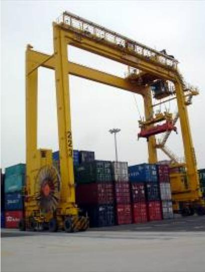
*BU: Motor cable reel represent a suitable alternative for the electrification of RTGs.*
