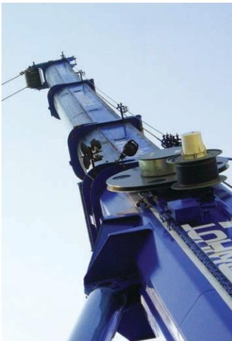
Slip ring assembly in construction machine
