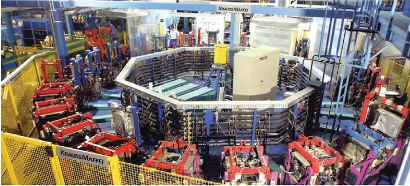
Rotary injection-molding machine from Krauss-Maffei Kunststofftechnik (Munich)
