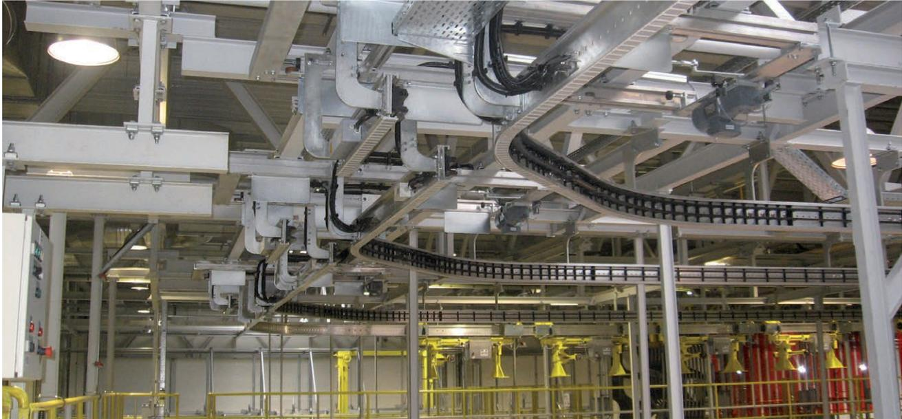
When supplying power to rail guided vehicles, a continuous inductive supply is generally required along the entire path of travel. The IPT® primary track is installed parallel to the rail. The pickup is attached to the driven vehicle itself. In some cases trailer vehicles may be used.
