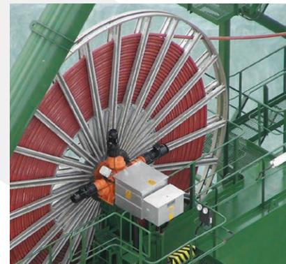
Medium-voltage motorized cable reel with magnetic coupler
