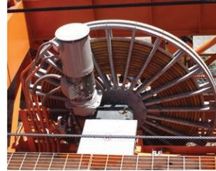
Motorized cable reel for spreader with variable frequency drive
