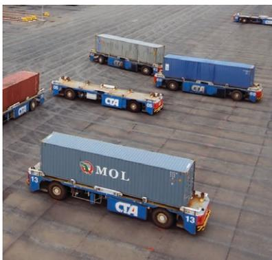
Fully automated AGV with electrical drives
