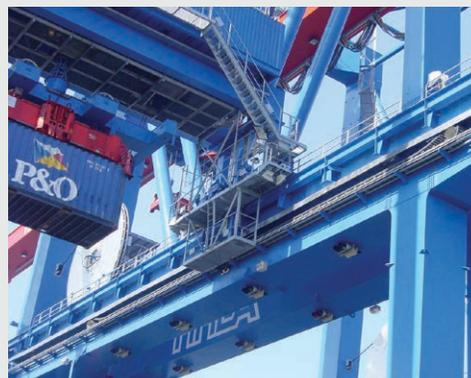
Cable chain system on a trolley – Hamburg, Germany
