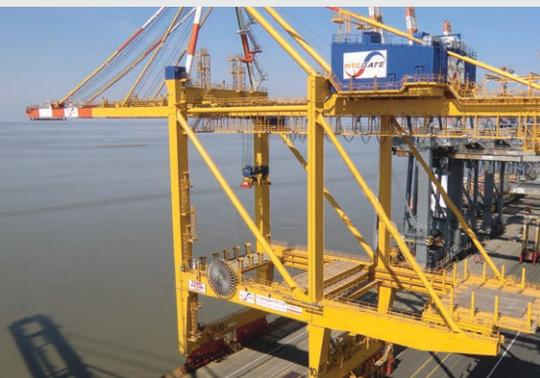
High-speed festoon system on a ship-to-shore container crane
