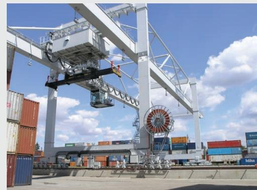
Standard festoon system and motorized cable reel on an intermodal crane
