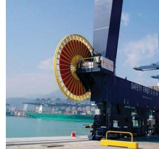
Medium-voltage motorized cable reel on STS Crane at YICT in China
