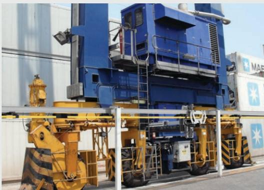
Conductor Rail "Drive-In" System for E-RTG
