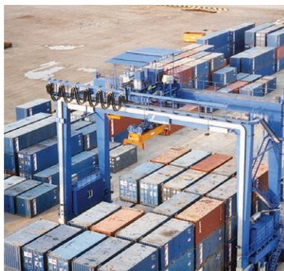
Standard festoon system for RTG-Main trolley
