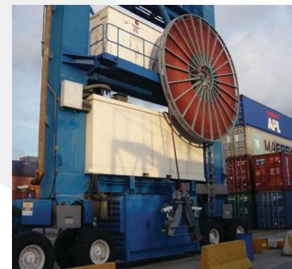
E-RTG (Plug-in-version) with cable reel solution
