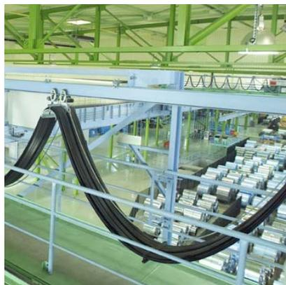
Energy and data transmission on a steel-mill-crane
