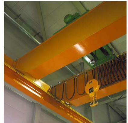
Power supply of the crab on an overhead bridge crane
